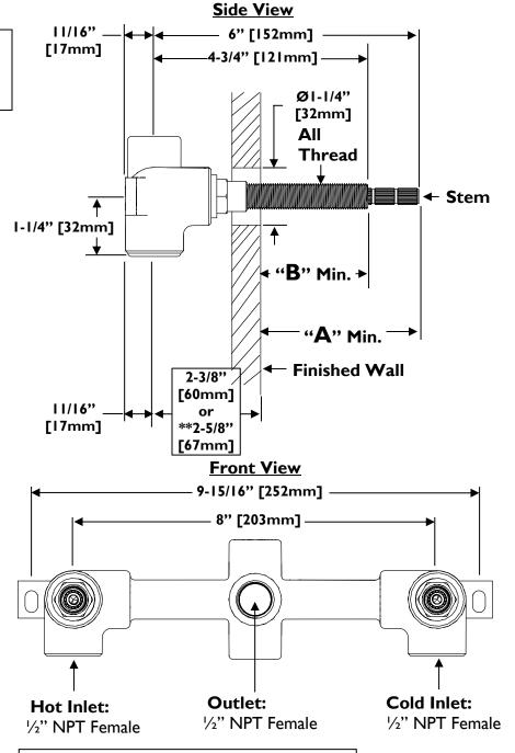
**\*\*\*NOTE:** Valve rough must be set back a minimum of 2-5/8" [67mm] from finished wall surface to center of inlets
